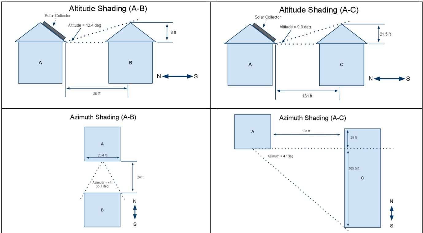
Figure 2: Shading calculations for building B and C.
