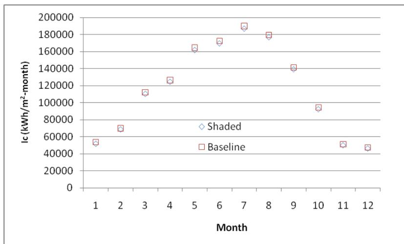
Figure 3: Monthly radiation incident on collector before and after shading analysis.
