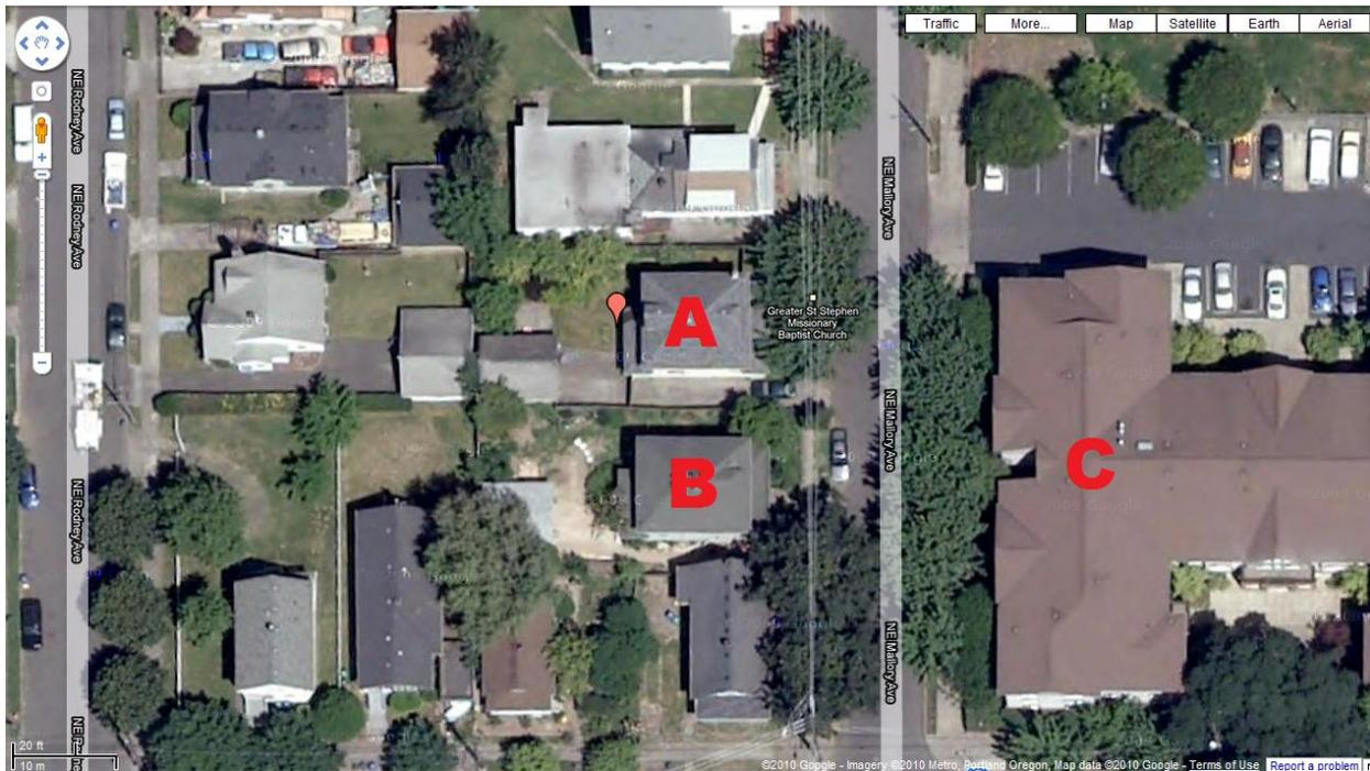
Figure 1: Site context of residence. Building A is residence, buildings B and C are tall enough to shade the roof of building A.
