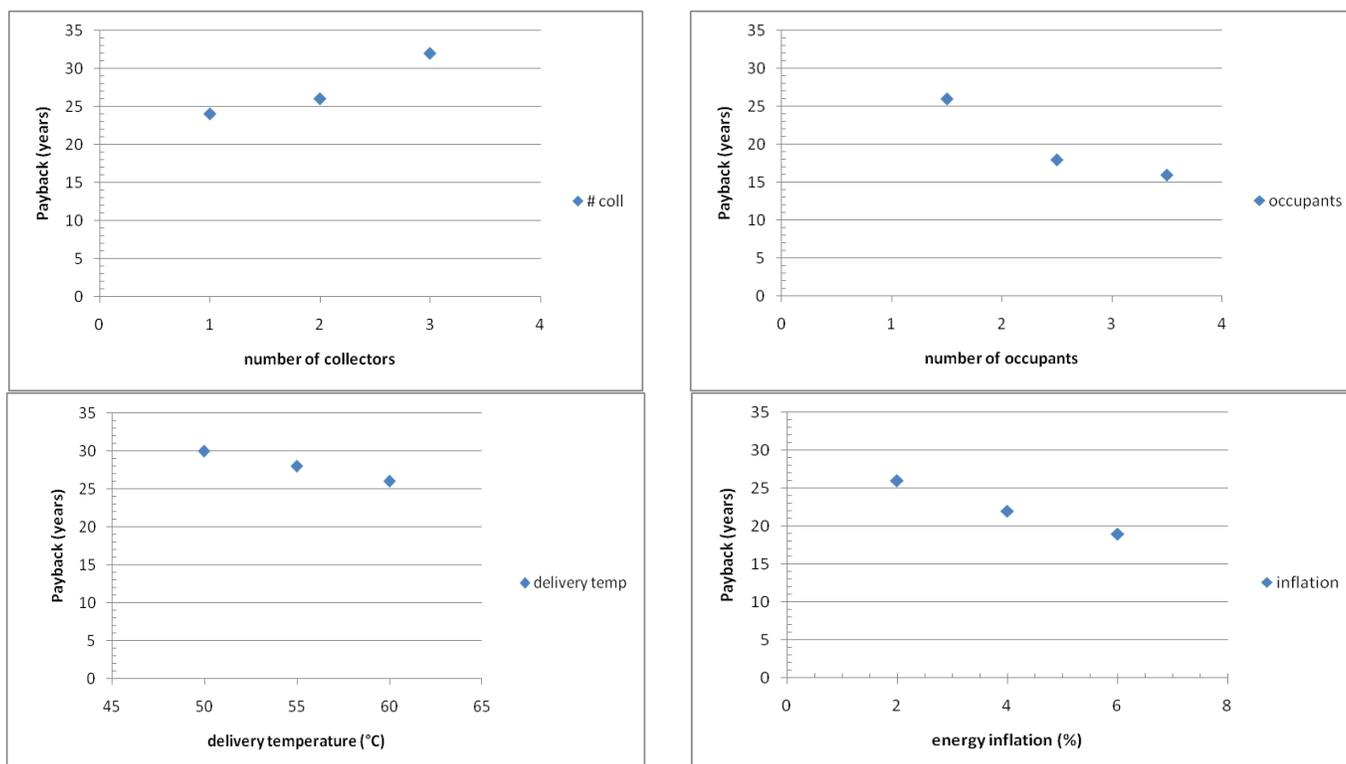
Figure 4: Sensitivity of payback period to number of collectors, occupancy, delivery temperature and energy inflation rate.
