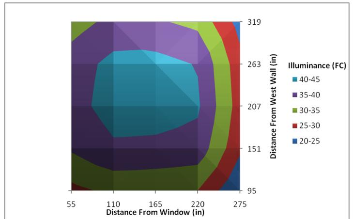
Figure 5: Measured illuminance of classroom with full artificial light conditions.
