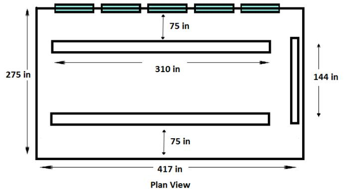
Figure 2: Shattuck Hall Room 211 luminaire placement. The long luminaires provide primary lighting for the room, while a short task light on the East wall provides illumination for the white board.
