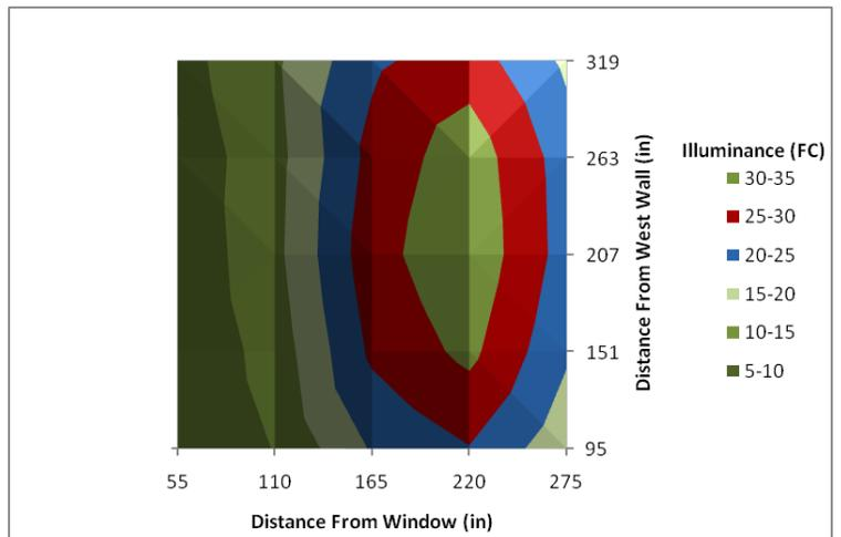
Figure 6: Measured Illuminance of classroom with only the luminaires on the South wall and East wall task lighting turned on.
