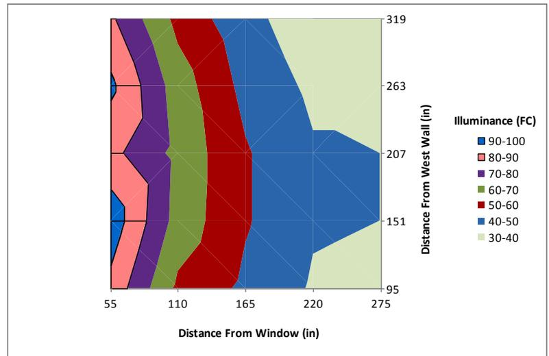
Figure 3: Measured illuminance due to daylight in classroom.
