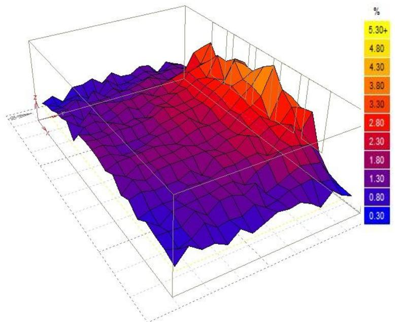
Figure 4: Ecotect model results showing daylight factor calculated for overcast conditions.
