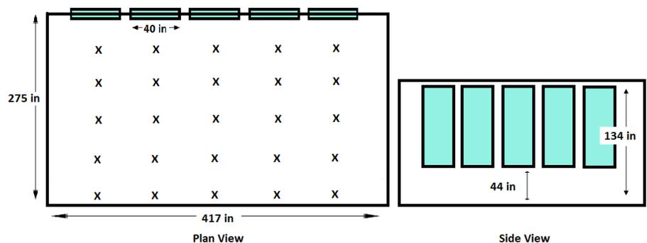
Figure 1: Shattuck Hall Room 211 window position and general layout. Measurements were taken at locations marked with an X.
