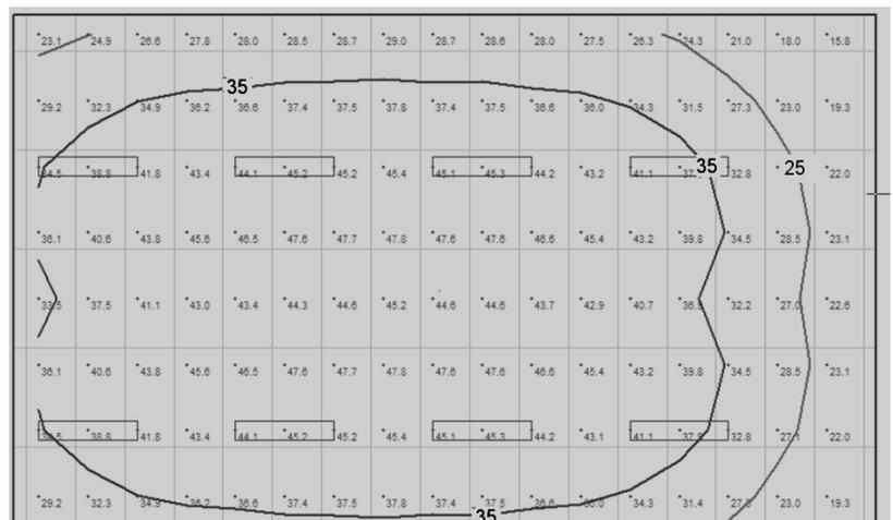
Figure 7: Classroom illuminance levels modeled with Visual Basic software.
